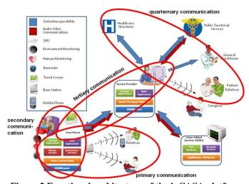
Figure 2 Functional architecture of the inCASA platform
