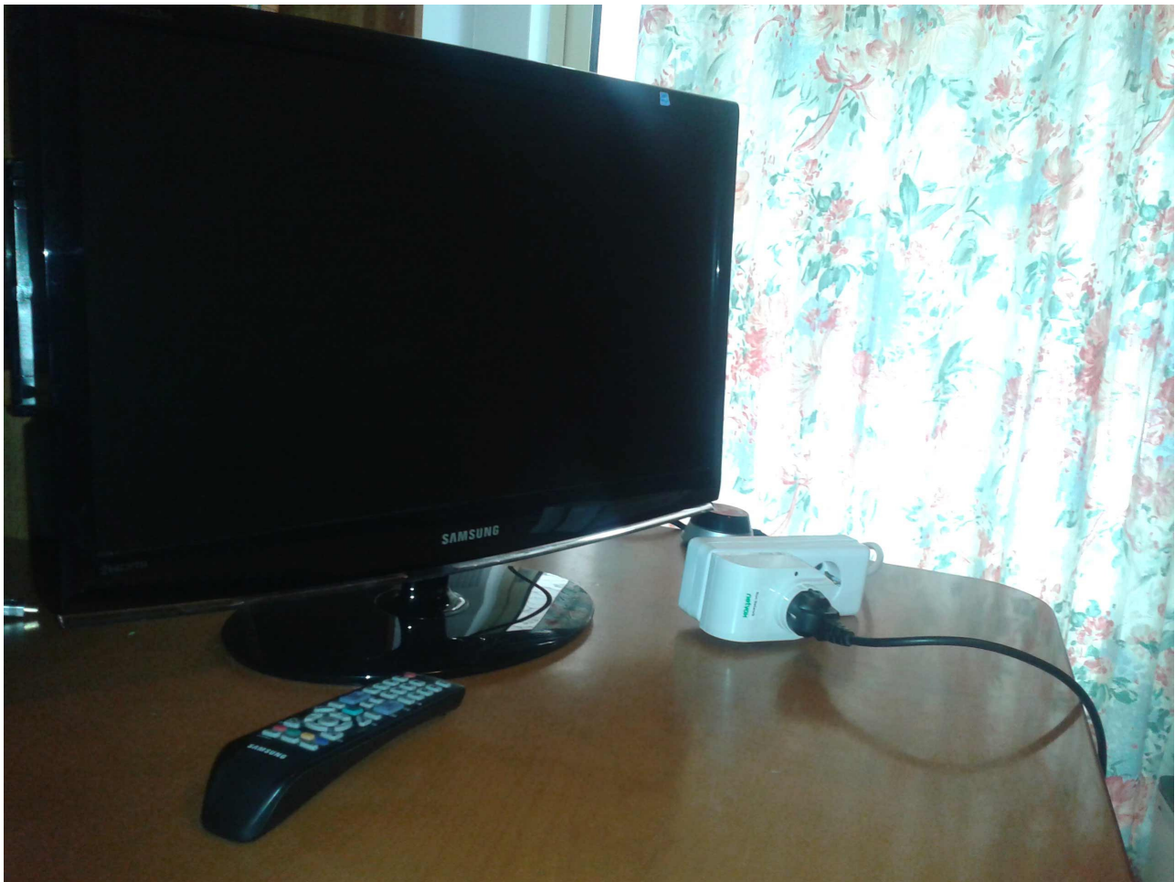
Figure 34 TV usage sensor connection
